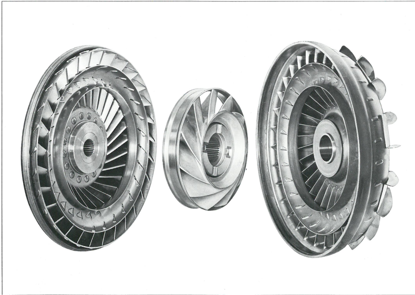
Fig. 2: The main components of the torque converter, from right to left: Impeller, stator, turbine.
