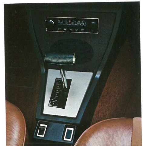
Fig. 4: Selector lever of ZF automatic transmission in two different makes of car
